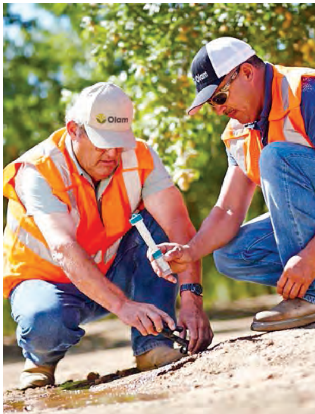
Collecting water samples directly from the California almond orchard drip lines to test for overall water quality.
